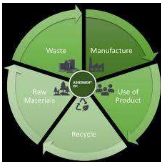
Figure 5.3 Circular cradle-to-grave Life Cycle Assessment (LCA) framework for a nanocomposite product: five interconnected stages — Raw Materials extraction → Manufacture (synthesis, fabrication) → Use of Product (water treatment, filtration cycles) → Recycle (regeneration of adsorbent, magnetic recovery) → Waste management (disposal or upcycling) — are evaluated together at the centre in terms of environmental impact categories such as global warming potential (GWP), ecotoxicity, and resource depletion. The circular layout highlights that end-of-life options (regeneration, recycling, magnetic recovery of active phases, or upcycling of spent media) can significantly reduce the overall environmental burden compared to linear, single-use scenarios by lowering demand for virgin raw materials and mitigating waste emissions. In the context of this manual, the figure operationalizes the sustainability concepts introduced in Chapter 5 by showing how nanocomposite-based water treatment technologies should be designed and assessed not only for high removal efficiency, but also for realistic service lifetime, ease of regeneration, and environmentally sound end-of-life management, aligning materials selection and process design with circular-economy principles. [Ramadan, B.S. et al. Circular life cycle assessment of nanocomposite-based water treatment technologies. Global NEST Journal , 2024, 26(7), 06216, Fig. 1. doi:10.30955/gnj.006216]
